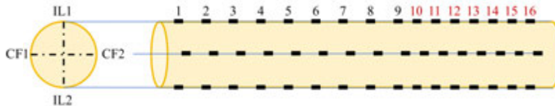
图5 光纤光栅应变传感器布置示意 Fig. 5 Schematic of Fiber Bragg Grating Strain Sensor Layout
