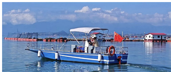
图 2 应用高温甲醇燃料电池的渔辅船 Fig. 2 Fishing Auxiliary Vessel Equipped with a High-Temperature Methanol Fuel Cell
