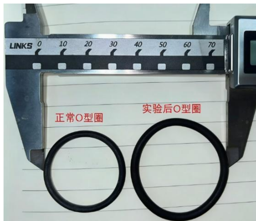
图 6 氢化丁腈材质 O 形圈试验情况 Fig.6 Experimental results of the hydrogenated nitrile rubber (HNBR) O-ring
